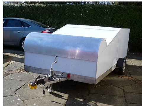
The trailer is lightweight to easily tow behind a normal saloon and is clad in aluminium with a hinged cover over the wheel rack.
